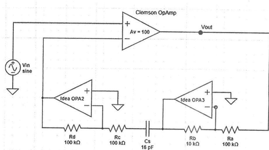
2. (20 points) There are two OpAmps., which are the OPA with an open-loop gain of 100 V/V and the OPA one is considered ideal listed in the following figure. Please determine the closed loop gain.
