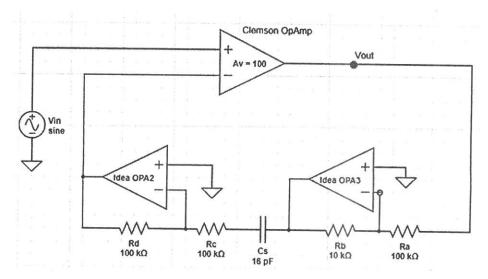
2. (20 points) There are two OpAmps., which are the OPA with an open-loop gain of 100 V/V and the OPA one is considered ideal listed in the following figure. Please determine the closed loop gain.
